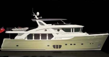
**CHINA** 75' Selene Ocean Explorer. Guido de Groot Design. Full Displacement w/ bulbous bow. Single or Twin Engine packages. 4 S/R + full crew.
