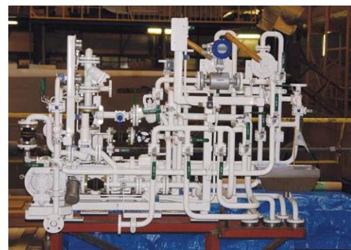
**ABOVE:** A few weeks after our visit, the 203' *Baton Rouge* underwent sea trials; Icon Yachts has perfected a modular type of constructions; entire sections of the engine room and piping are fully designed, painted and assembled outside of the hull, helping to streamline the build process
