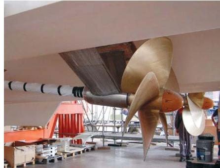
between the propeller blade tips and the hull bottom. Before the props are installed, have them balanced dynamically, not statically. That will minimize noise.
